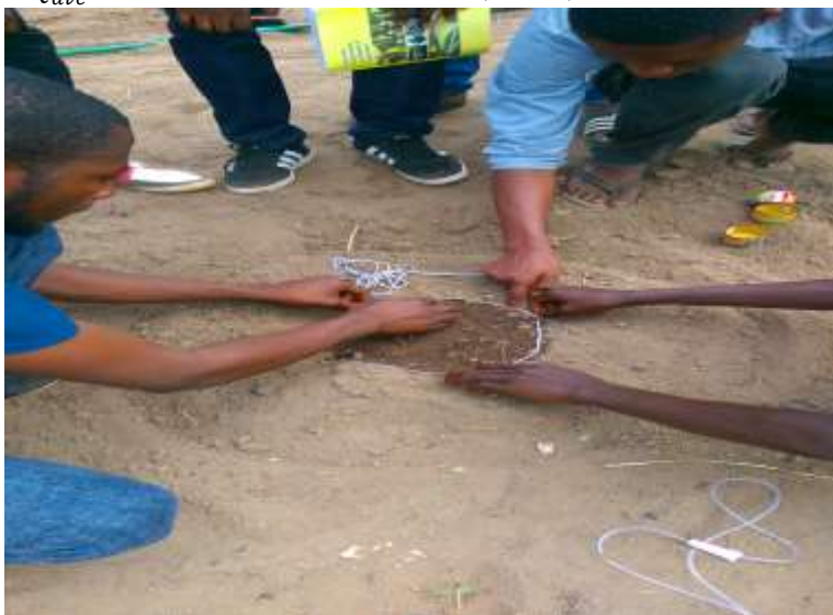
Plate.2. Determination of radius of wetted surface using planimetry method.
